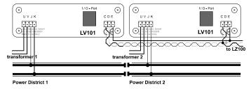
Figure 4 Connecting track voltage when using 2 LV101
