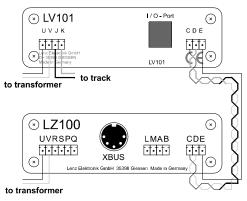
Figure 1 Connecting LV101 to Command Station LZ100
