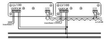
Figure 5 Connecting track voltage for large scale railroads
