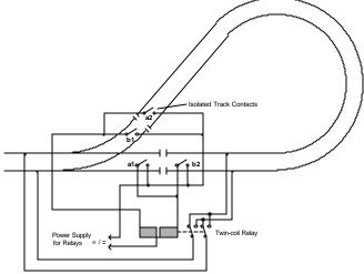
Figure 6: Wiring of Reverse Loops
