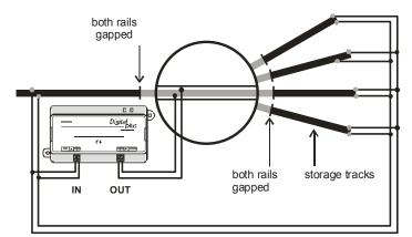
Figure 11: Wiring a turntable
