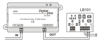
Figure 6: Connecting the LB101 to the LK200
