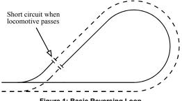
Figure 1: Basic Reversing Loop
