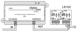
Figure 2: Connecting the LB100 to the LK200
