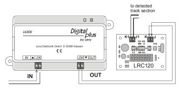
Figure 7: Connecting the LRC120 to the LK200
