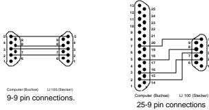
Both connections are shown from the soldering side.
