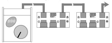
Some XpressNET systems do not have a RJ14 port. In this case simply connect the LA152 adapter using the LMAB connections.
