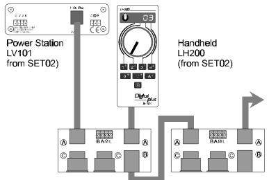
The master LH200 can then be connected to the second LA152 Port **A**. Other LH200s, LH100 or any other XpressNET devices can be connected to port **B**, **C**, or the **LMAB** connections. If you desire to plug in the master LH200 to a different LH152 then you must use a six wire RJ12 phone cable, between the LA152 adapters. Otherwise you can use a less expensive RJ14 based four wire connector to interconnect your LA152 adapters.
