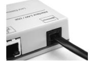
If you want to connect the Interface 23151 to the terminal screws LMAB of a LZ100/LZV100 command station, simply cut the cable in the middle and connect the cable wires to the corresponding terminal screws. The pin assignment is shown in the illustration on the right.
