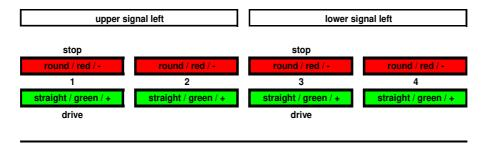
The two signals with 2 lamps each at the right clamp bar can be controlled separately via the decoder addresses 5 and 7:
